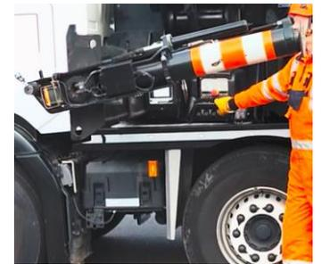
Swing-up stabiliser rotating away from Operator on opposite side of vehicle (manufacturer dependent)
